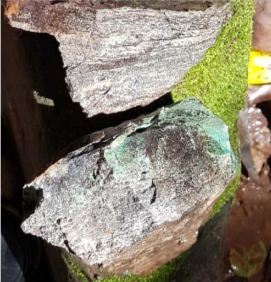
Photo 2: Sample TC190526. White quartzitic sandstone with disseminated bitumen and secondary copper minerals. 2.5% Cu and 36 g/t Ag.
