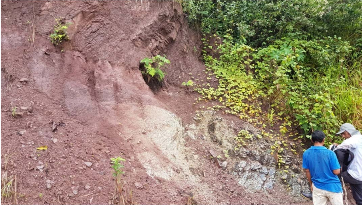
Photo 2: Sample TC190526. White quartzitic sandstone with disseminated bitumen and secondary copper minerals. 2.5% Cu and 36 g/t Ag.
