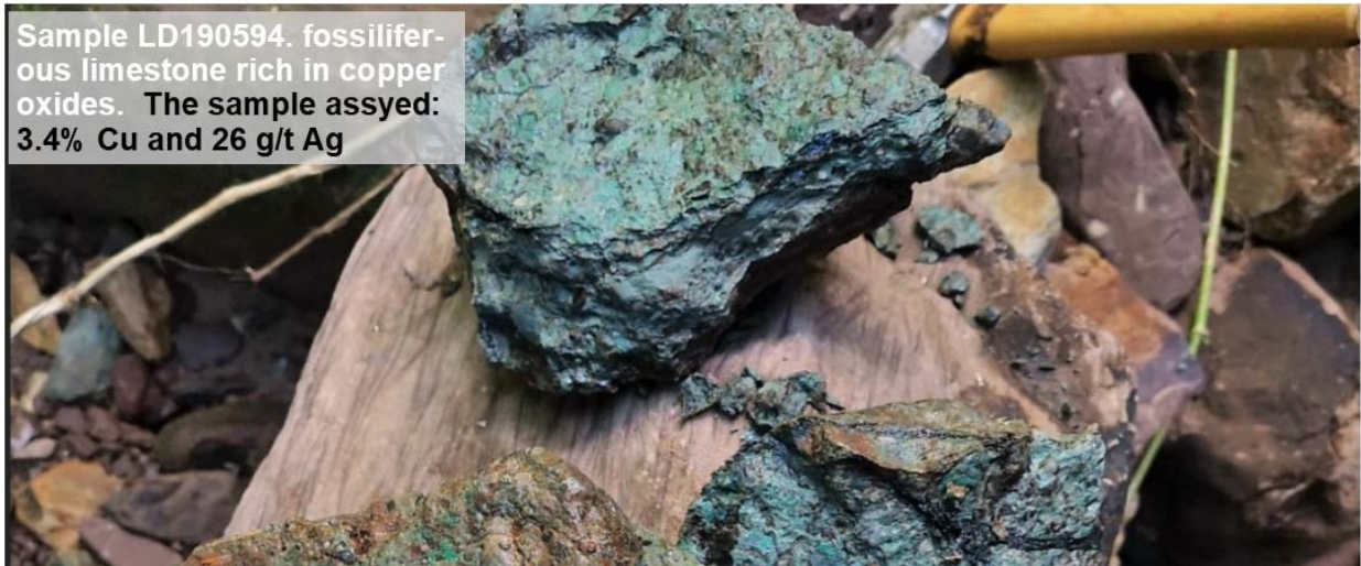
Figure 6. Photos of mineralized float discovered at Sacanche. Demonstrating copper mineralization in other lithologies than what has been discovered in outcrop too date.
