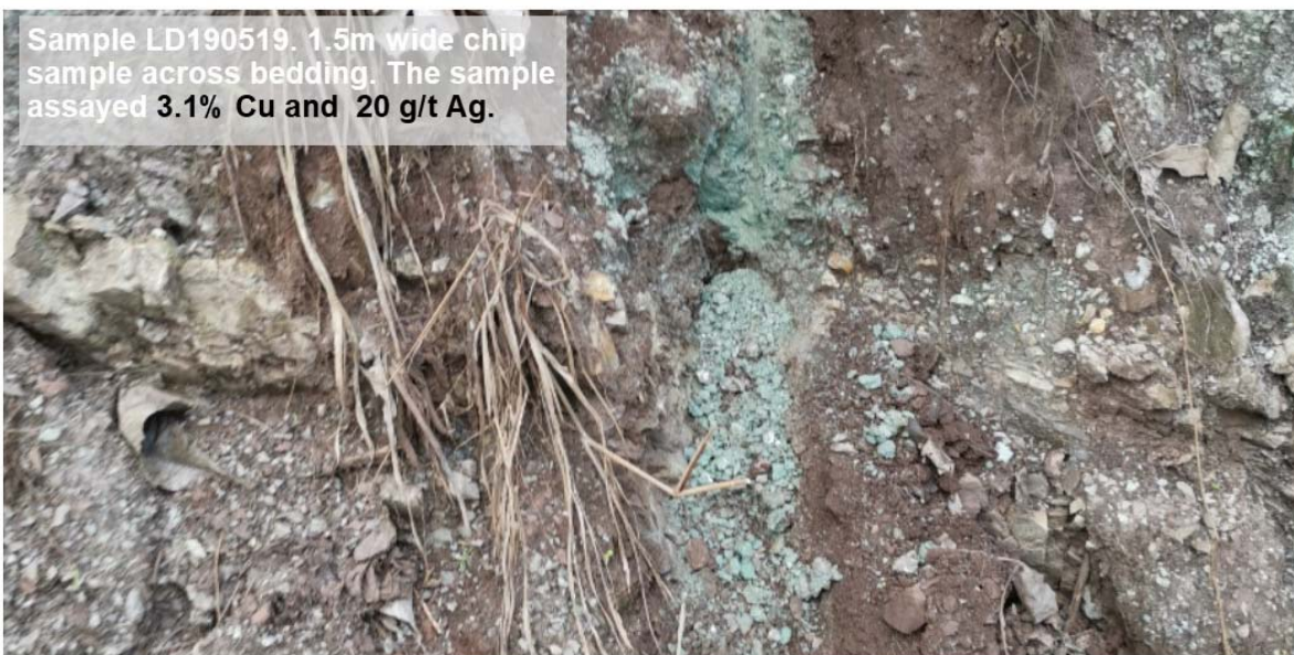
Figure 5. Photos from mineralized outcrop at Sacanche. The outcrop consists of bleached siltstone with fine lamination of plant carbon in bedding planes. Three continuous and representative chip samples across bedding. The zone assayed: 3m @ 2.5% Cu and 22g/t Ag . The greater zone is 5m wide and assayed: 5m @ 1.7% Cu and 14g/t Ag
