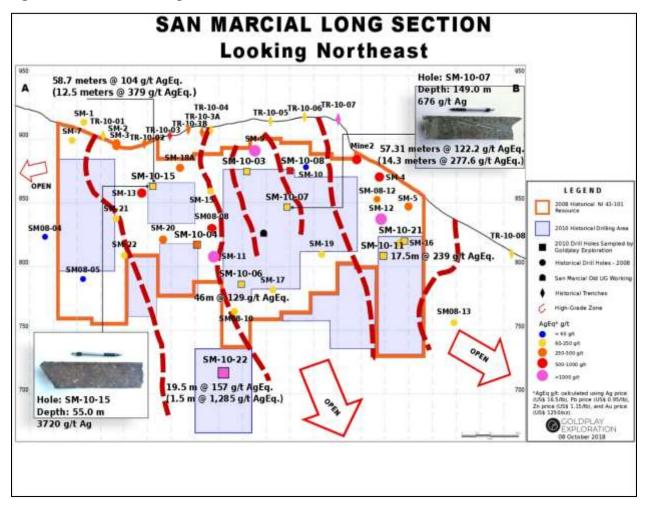
Figure 4: San Marcial Longitudinal Section A-B
