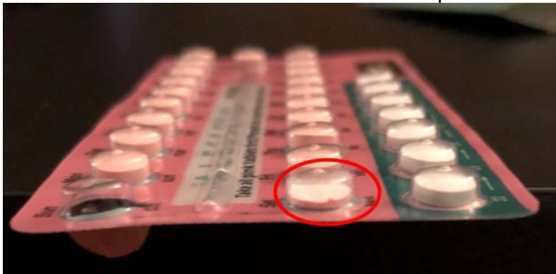
Side view of Alesse 28 blister back with broken pill circled in red
