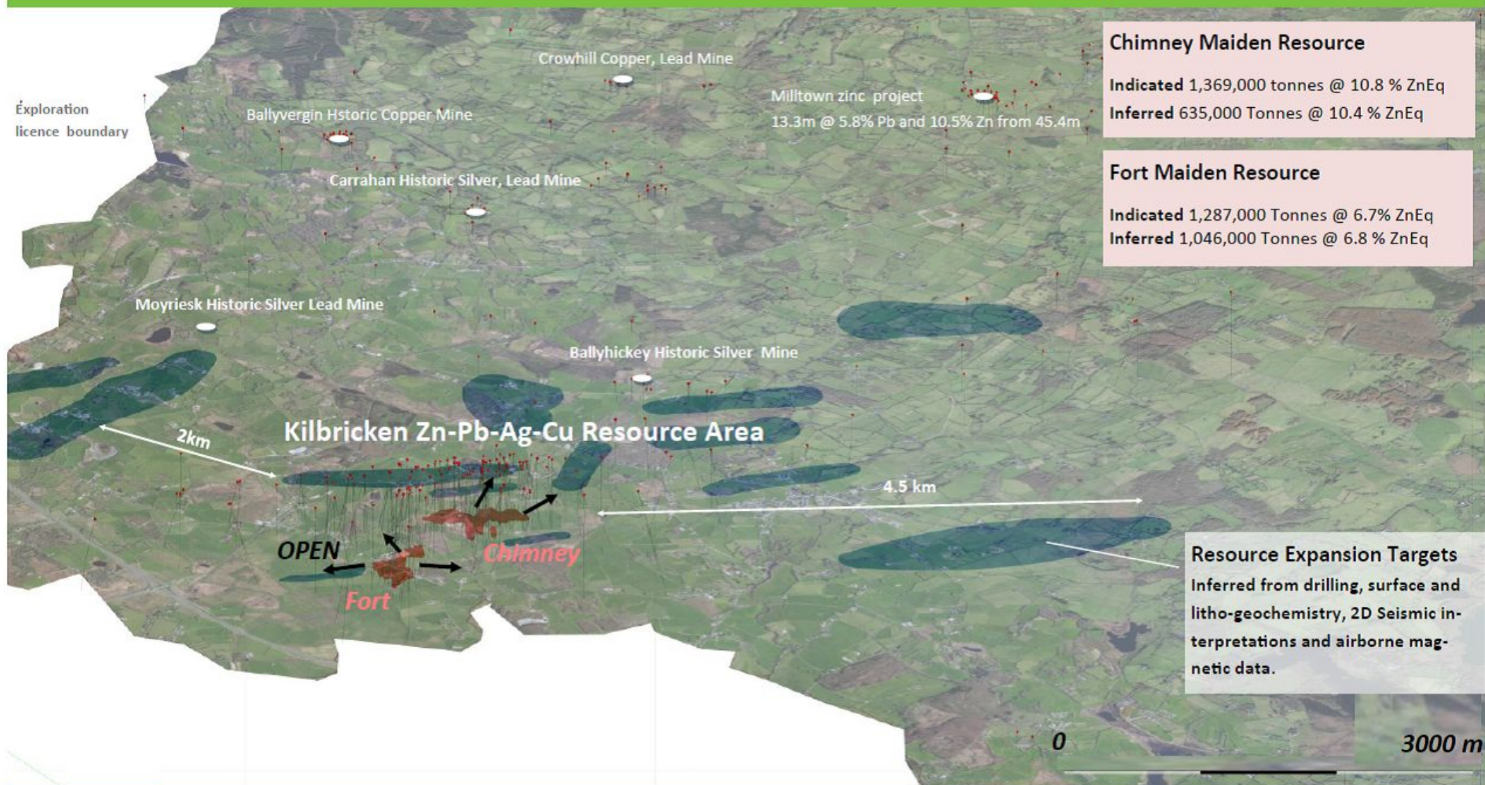
Figure 2 — Regional Kilbricken Area: Inclined view looking north east showing resource area, resource expansion targets, diamond holes and historic prospects.
