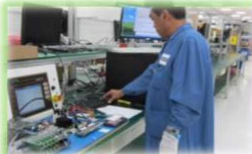
SBC FUNCTIONAL TESTING
