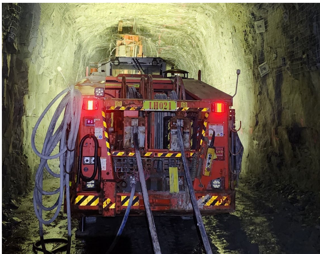
Figure 5 – Long Hole rig drilling the first South Junction stope
