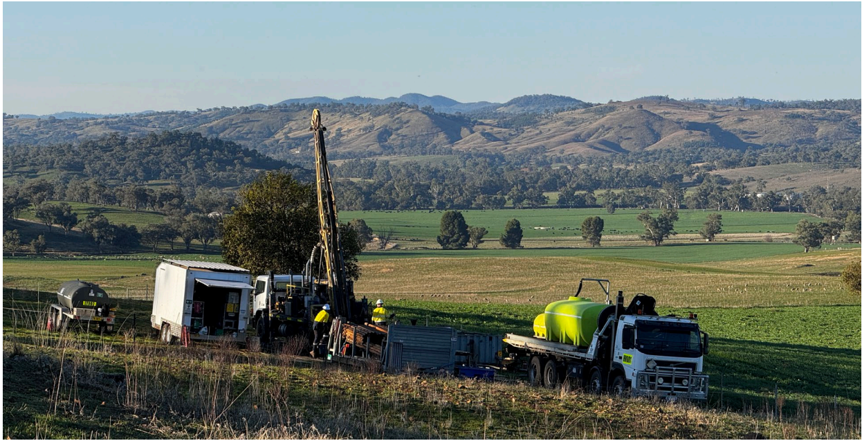
Figure 3: Earth AI's low cost Mobile Low Disturbance (“MLD”) diamond rig in operations at Cundumbul drilling hole ECU18D
