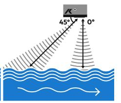
KISTERS' HyQuant L sensor uses FMCW technology in the 60 GHz frequency band for water level measurement without direct contact. The HyQuant L radar water level sensor is compact, lightweight and IP68-rated with a narrow beam width, high precision, and built-in filter algorithms.
