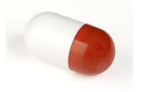
This condensed technology communicated in real time at a frequency of 30 seconds with a dedicated monitor, the eViewer Medical, which records the data autonomously and triggers alerts if the threshold is exceeded. The temperature is accurate to within  $\pm 0.1^{\circ}$ C of the human physiological range between 36-41°C, and the communication protocol guarantees data security.
