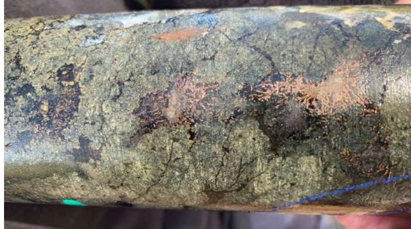
Native copper, chalcocite, chalcopyrite and black chlorite in skarn: 4.24g/t gold & 1.6% copper @ 60.6-61.6m
