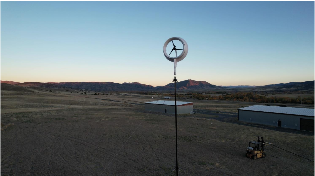
Image: HFI’s 1 metre diameter prototype wind energy hydrogen production system undergoing testing in Montana, USA (October 2022)
