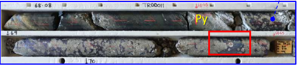
ABOVE - TRDD011: Skarn zone massive sulphide with bornite (Bn) and pyrite replacing garnet within 14m @ 1.39 g/t Au, 1.69% Cu from 58m, including 4m @ 3.36 g/t Au, 4.98 % Cu from 68m (right).
