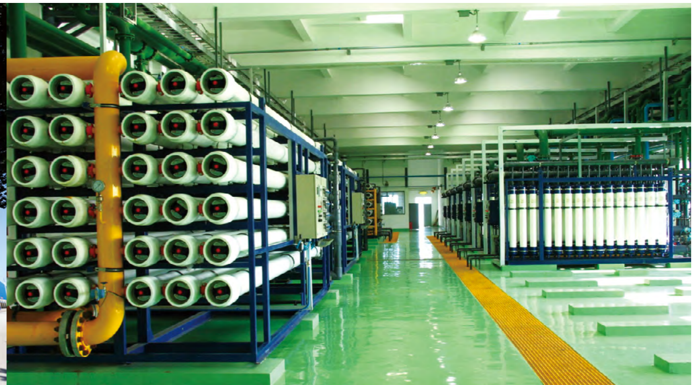
Hebei Wangtan Power Generation Company steps up efforts in freshwater production through seawater desalination, saving more than 500,000 tons of tap water annually.
