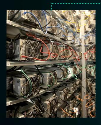
Mining requires application-specific integrated circuits ("ASICs") – advanced computers customized for bitcoin mining
