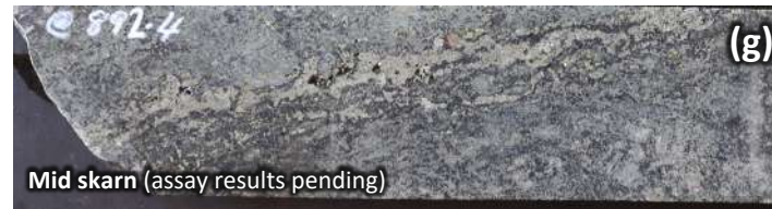
(g) Garnet-magnetite-pyrite and disseminated chalcopyrite
