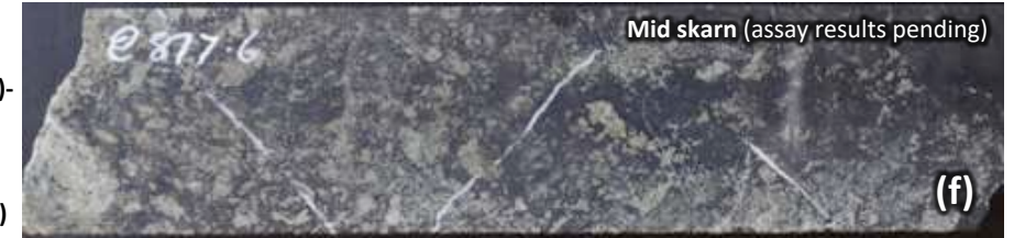
(f) Predominantly with magnetite (black)-garnet (olive)-disseminated pyrite (dark yellow) & disseminated chalcopyrite (yellow)
