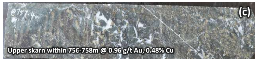
(b) & (c) Prograde garnet (olive)-magnetite (black)-pyrite (dark yellow)-chalcopyrite (yellow), cut by later retrograde carbonate (tan iron carbonate & white calcite)-hematite (red)-chalcopyrite (yellow).
