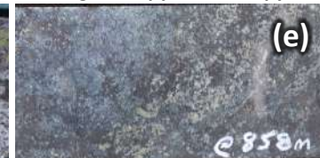
(e) Middle Skarn with garnet-magnetite-pyrite-chalcopyrite
