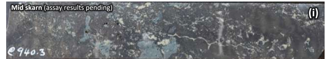
(i) magnetite (black)-garnet (olive)-disseminated pyrite (dark yellow) & disseminated chalcopyrite (yellow)
