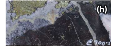
(h) magnetite-garnet-pyrite-chalcopyrite, cut by iron carbonate-calcite with large clots of chalcopyrite
