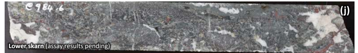
(j) developed in crystalline limestone (light-grey) with disseminated magnetite (black)-pyrite (dark yellow)-& hematite (red) along with later carbonate fill (white)
