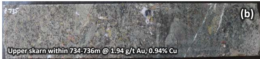
(b) & (c) Prograde garnet (olive)-magnetite (black)-pyrite (dark yellow)-chalcopyrite (yellow), cut by later retrograde carbonate (tan iron carbonate & white calcite)-hematite (red)-chalcopyrite (yellow).
