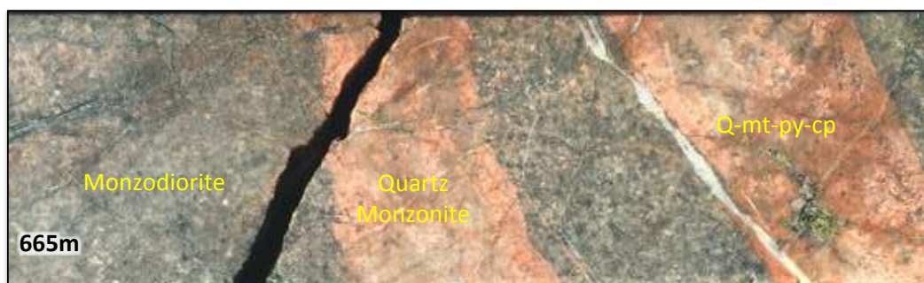
Grey monzodiorite (crowded) with albite alteration cut by red quartz monzodiorite vein dykes containing examples with clots and veinlets with quartz (Q) +/- magnetite (mt) +/- pyrite (py) +/- chalcopyrite (cpy) (at 665m downhole).
