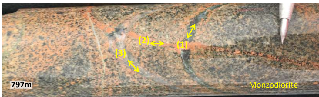
Monzodiorite (crowded) with albite alteration and hematite dusting cut by vein sets comprising: (1) early quartz-magnetite, then (2) kfeldspar (orange-red)-pyrite and (3) later quartz-pyrite (at 797m downhole).
