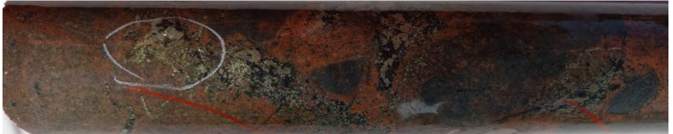
(c) Monzonite dyke network (red-orange) cutting monzodiorite (grey) with pyrite, magnetite and chalcopyrite and interpreted potassic alteration along the contacts in a section at 720.5m: 2m @ 0.62g/t gold, 0.10% copper and 11ppm molybdenum and within a broader zone of 18m @ 0.75 g/t gold, 0.09% copper and 14ppm molybdenum from 712m
