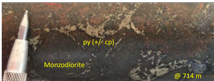
(d) LHS: Monzodiorite (grey) cut by monzonite (red-orange) in an interval with: 2m @ 0.91g/t gold, 0.12% copper & 19ppm molybdenum (from 714m); and, RHS: Monzodiorite (grey) cut by monzonite (red-orange) in an interval with 2m @ 0.47g/t gold, 0.06% copper & 17ppm molybdenum (from 718m).
