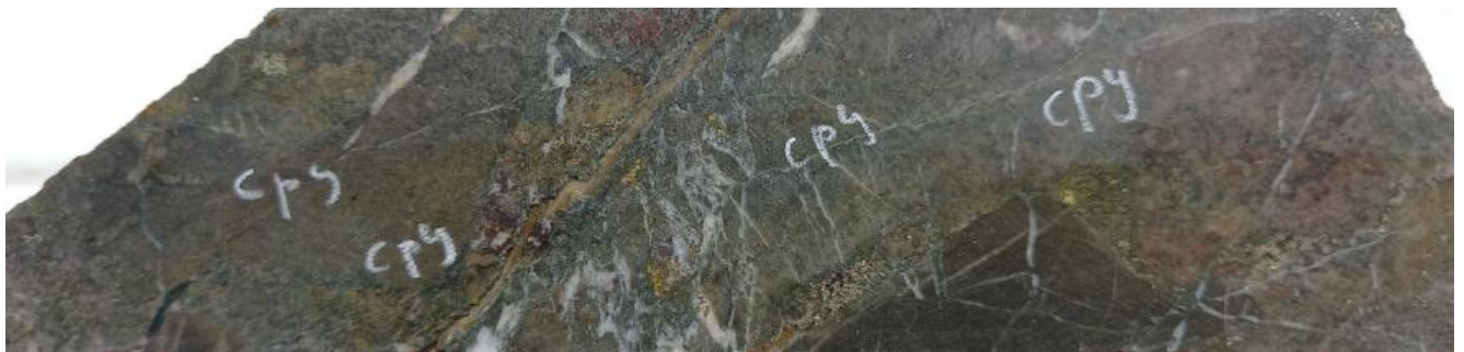
(e) Disseminated chalcopyrite around pyrite at 728.8m: 2m @ 1.03g/t gold, 0.15% copper & 15ppm molybdenum
