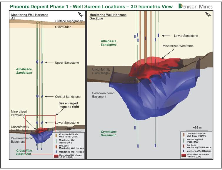
Figure 2: 3D Isometric Views of the Phoenix Deposit (Phase 1) – ISR Test Pattern Showing Locations of Monitoring Well Horizons
