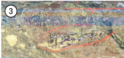
196.2m Vein hosted bornite & chalcopyrite
