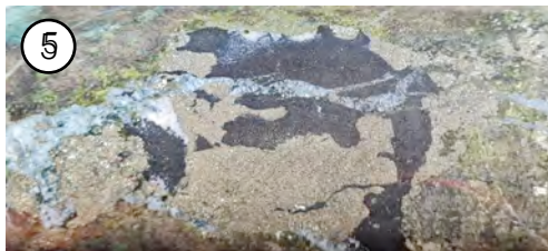
362.5m Pyrite, magnetite, chalcopyrite & yellow garnet
