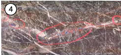
205.1m Vein hosted bornite, chalcopyrite & covellite
