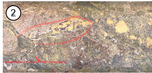
160m Vein hosted primary bornite and chalcopyrite
