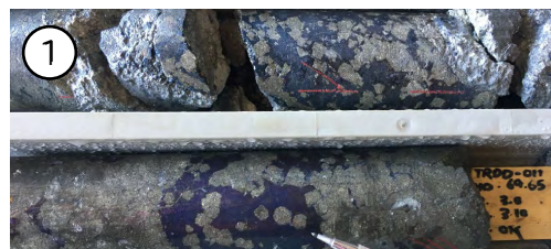
69.7m fault bounded coarse pyrite, covellite & chalcocite
