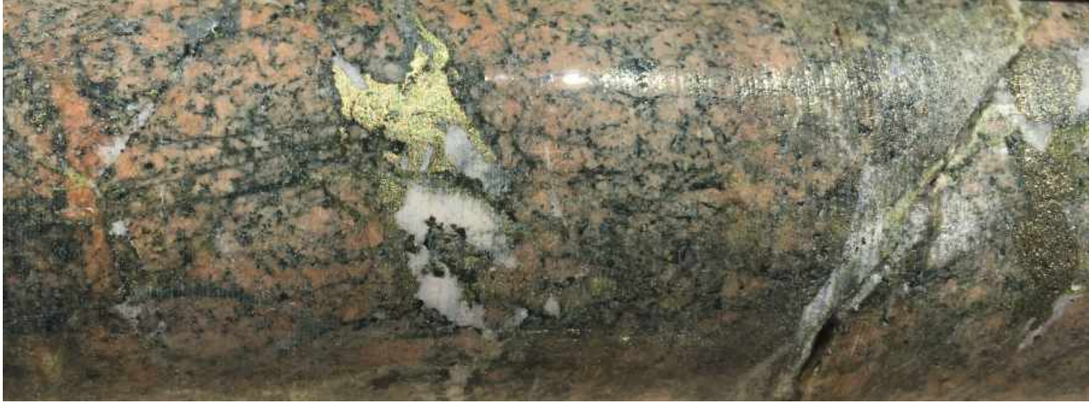
Pink-red altered monzonite cut by quartz vein with chalcopyrite Hole TRDD006, Mordialloc target at the Trundle project, Central West NSW, Australia
