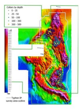
Typhoon survey chargeability with >14m sec iso-surfaces shown in grey (section >1km depth)
