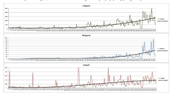
CTD006 assays showing increasing trend of copper (top), molybdenite (middle) and gold (bottom) down hole. Assay values in ppm. Scales: Cu, 0-2500ppm; Mo, 0-100ppm; Au, 0-0.25ppm (G/t)  $^{5}$
