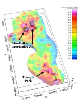
At the Trundle Park prospect mineralized intercepts are associated with magnetite skarn, similar in style to the Big Cadia skarn that is peripheral to the Cadia porphyry copper-gold deposits. Significant intercepts at the Trundle Park prospect include:
