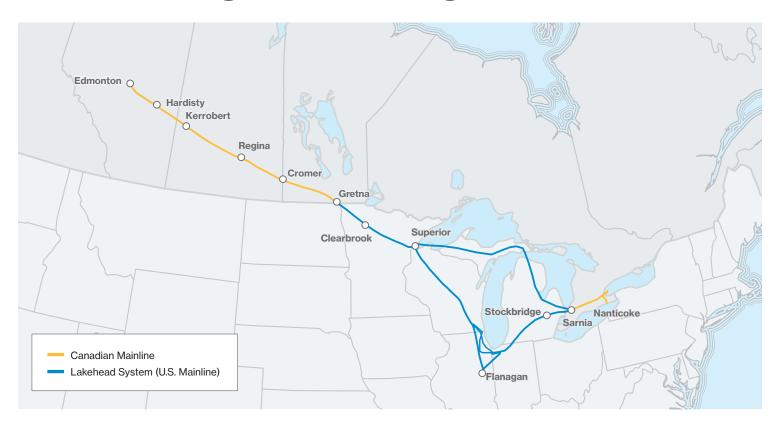
Enbridge operates the largest crude oil pipeline system in the world, and the Mainline is an integral part of that system. It includes five pipelines that begin in Edmonton, Alberta and cross the Canada – U.S. border near Gretna, Manitoba, where it operates in the U.S. as the Lakehead system. The current cross-border capacity of the Mainline is approximately 2.9 million bpd.
