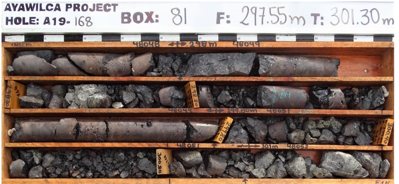
Figure 2. Drill core photograph from the high-grade lower interval in A19-168
